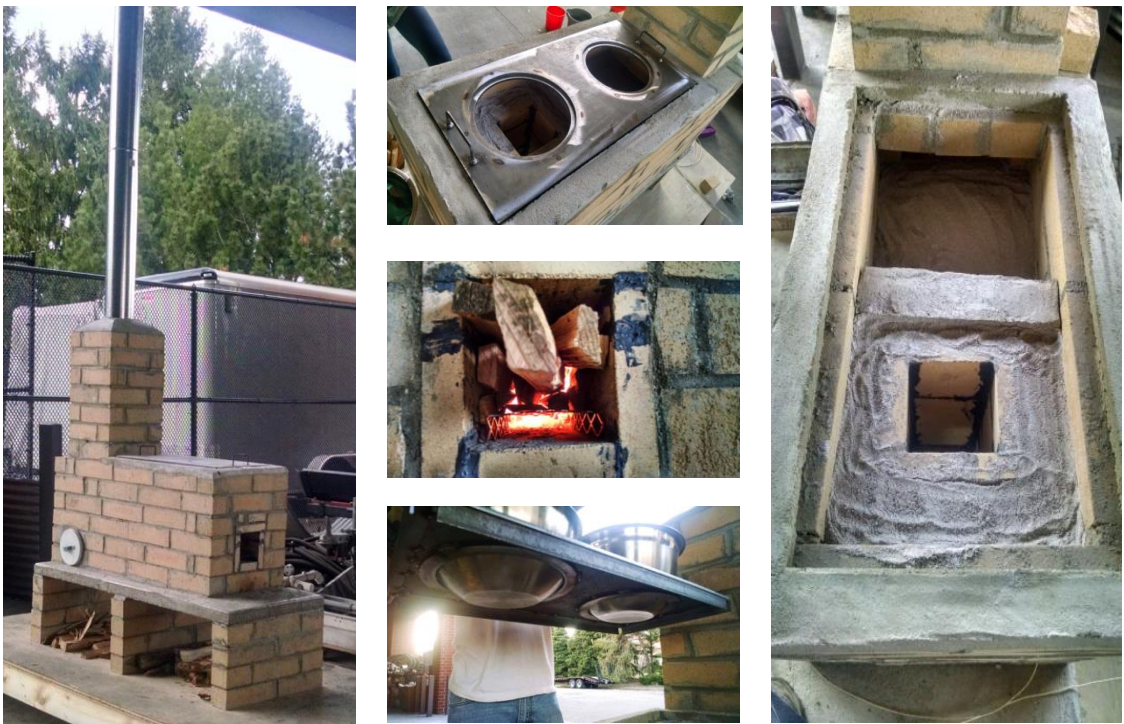
Left: Stove Body Center top: Steel cooking surface Center middle: Entrance to chamber showing grate Center bottom: Round bottom pots in steel cooking surface Right: Ash insulation of combustion chamber
